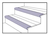
**Installation:** Measure and cut to fit. Use a sanding sponge to prepare floor and Stair Nose for adhesive. Remove backing paper from tape and affix Stair Nose using adhesive, being sure to follow adhesive manufacturer's instructions completely.
