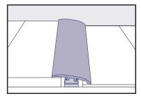
**3-N-1 as a Reducer:** Used to transition from a hard surface floor (PROCORE) to a floor with a lower height such as ceramic tile or vinyl.
