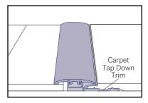
3-N-1 as an End Cap: Used for transitioning from a hard surface floor (PROCORE) to carpet.
